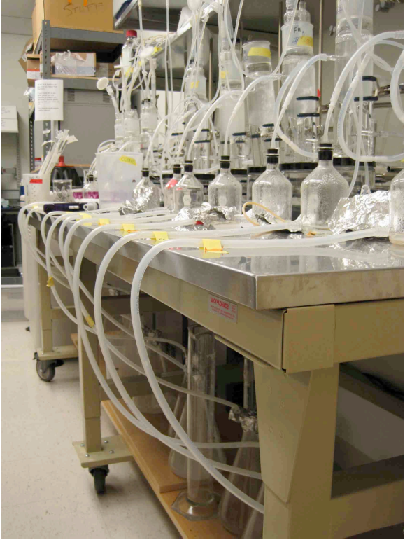
Figure 12. Downward angle of effluent track prevents contamination from reverse flow.
