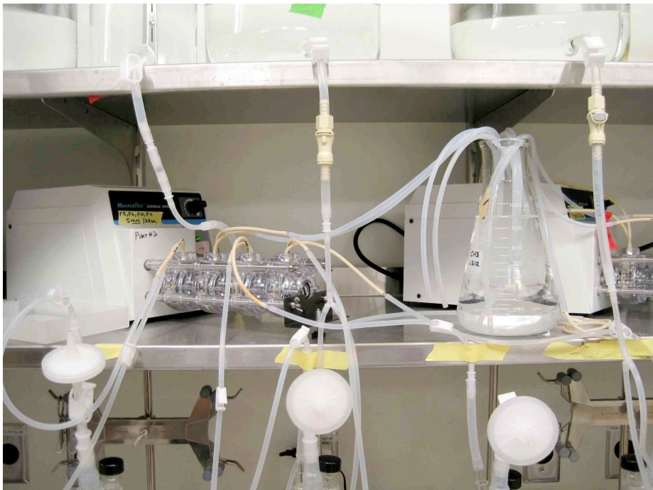
Figure 15. Dummy lines simulate active chemostat lines, so you don't have to adjust the pump.
