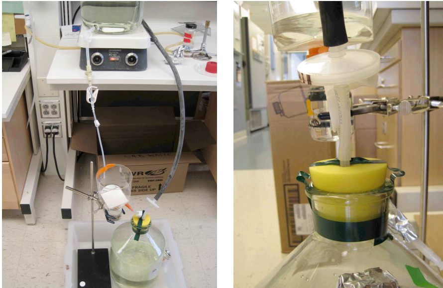
Figure 9. During filtration, it's normal for the cork to get slightly sucked in.
