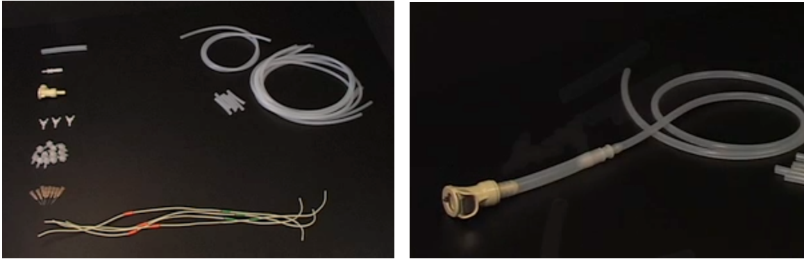
Figure 9: Media line parts and assembly of the quick-connect, which attaches to the media carboy.
