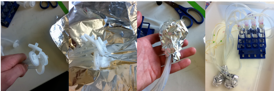
Figure 7: Preparing the air lines for the autoclave.
