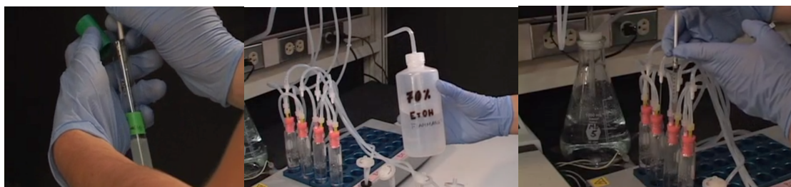
Figure 16: Inoculating the ministat
