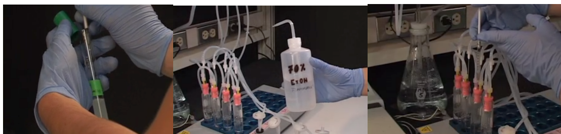
Figure 22: Inoculating the ministat.
